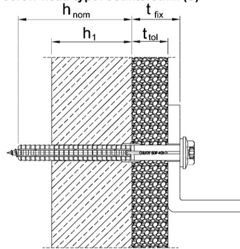
**Intended use SDF-10H in concrete/masonry/
