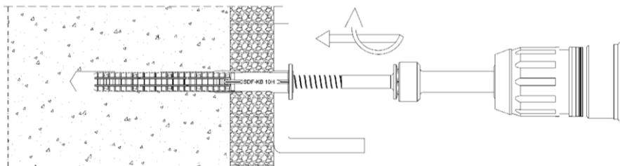
4. Correctly installed anchor
