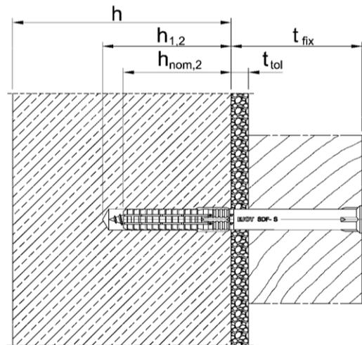
**Intended use SDF-10V in concrete ( $h_{nom1}$ )**
