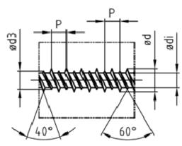
thread "E" alternative with rounded thread ground
