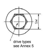
head "S" round pan head with thick shaft
