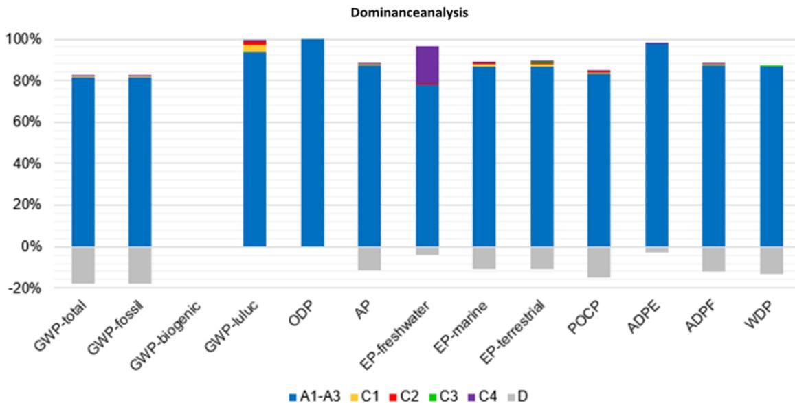
All indicators are significantly dominated by the production stage and the material and energy upstream chains (module A1-A3). In the A1-A3 module, the screws in particular
